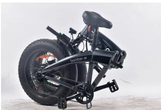
4. Bend the handlebar on the bicycle in order to complete the folding as shown in the photo alongside
