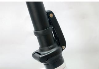
3. Unlock the safety hook on the handlebar
