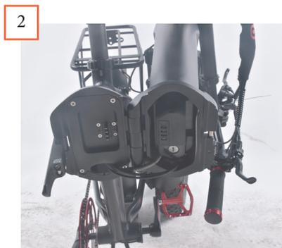
1. Open the bicycle frame by unlocking the safety lever (1).
