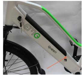
After charging is completed, pull out the charger plug from the socket, then disconnect the charger connector from the bicycle charging hole. Do not leave the charger connected to the socket for a long time after charging has been completed. If a smell comes out from the charger during charging, the temperature may have become too high; please stop charging immediately and send the unit for maintenance.
